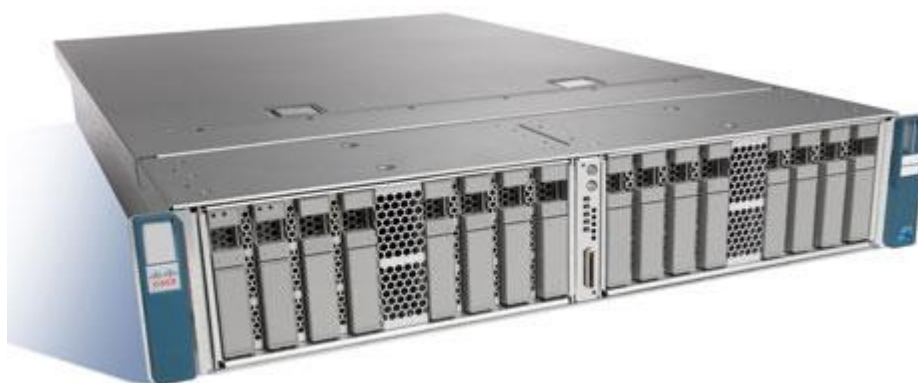
Figura 21. Cisco UCS C260 M2 Rack Server
