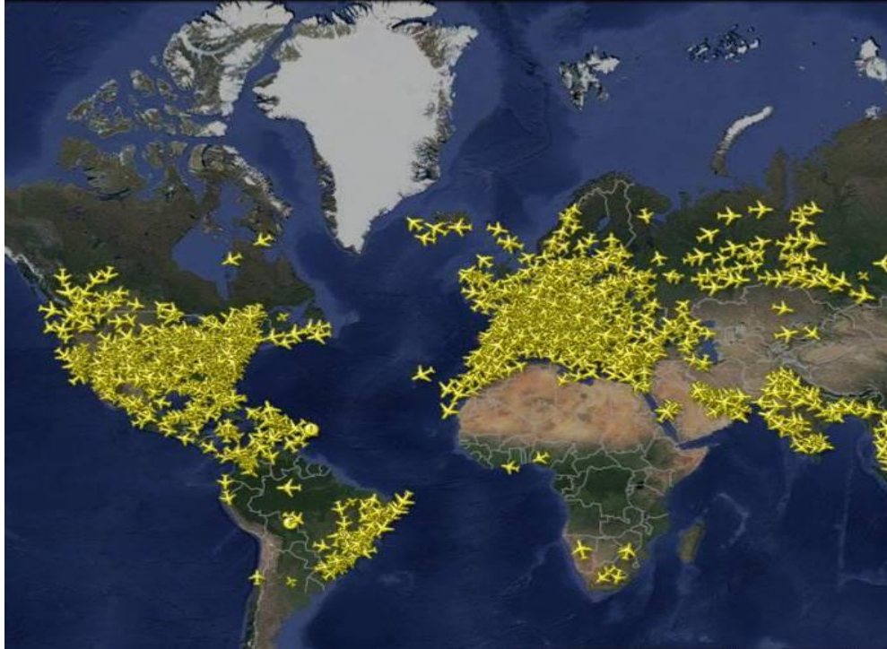
Figure 6. Coverage of terrestrial ADS-B system [20]
