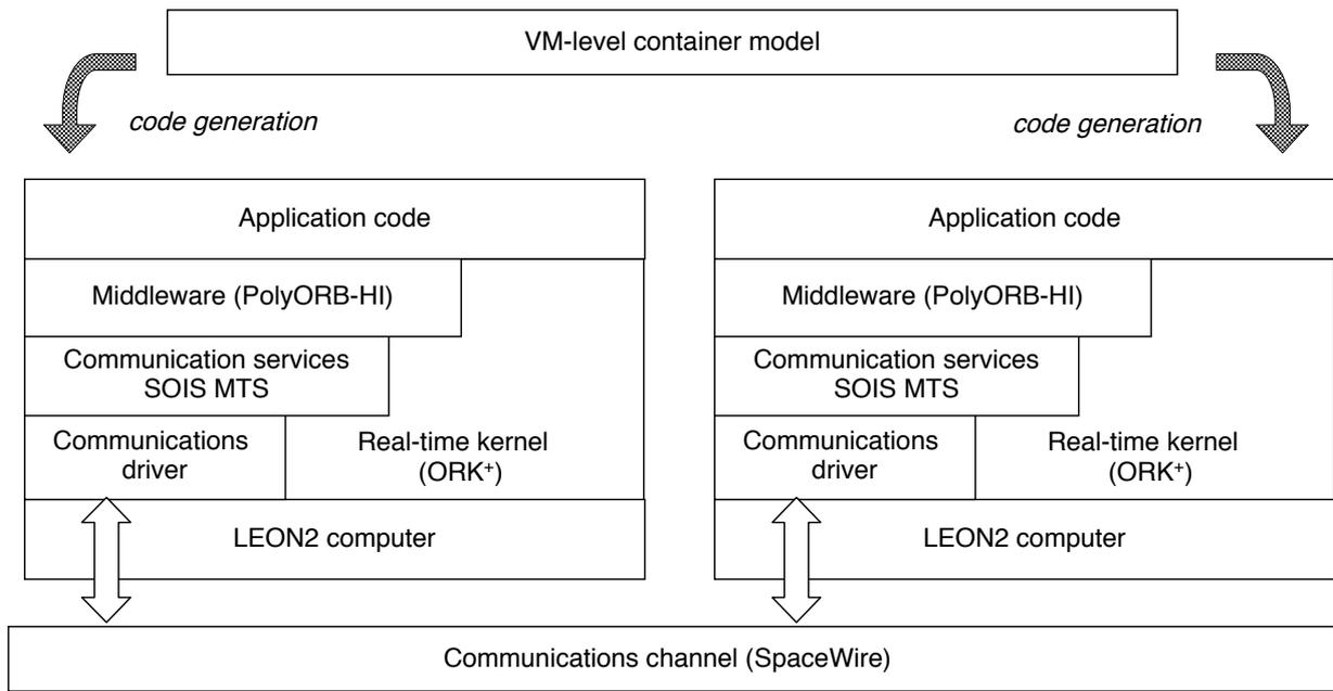
Figure 1. ASSERT Virtual Machine Architecture.
