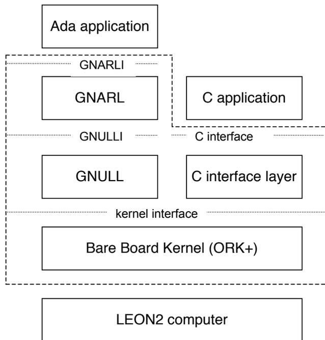
Figure 2. Architecture of the GNAT for LEON run-time system.
